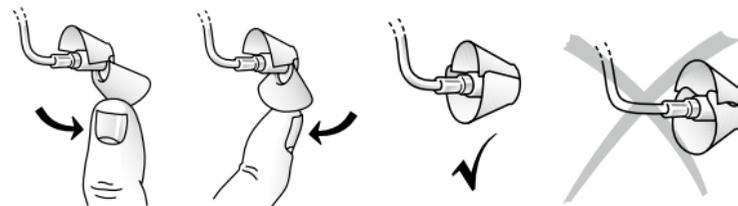
1. Push the largest petal away from the thin tube using a finger. This bends the petal forward.
